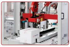
**BESTPACK'S "SOFT TOUCH" SYSTEM** Air powered belt drive and sealing section decreases product damage while maintaining presentation.
