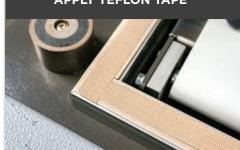
Then, use the 1/2" Teflon tape, placing it as centrally as possible on the seal pad.
