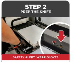
Heat your knife. You can do this by either activating the L-Bar by pressing down or pressing and holding the limit switch a few times.
