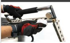
Use a clean cloth and raise the film clamp and wipe the knife for any excess plastic residue.
