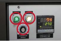
Turn on the shrink tunnel power and heater.
