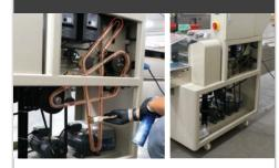
Using the paint brush, dip it in grease and apply to the chains from top to bottom located on the back of the machine.
