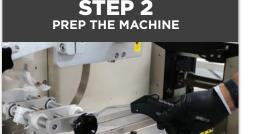
Use compressed air to blow all residue and build up off the machine.
