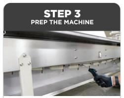
Unlatch bottom of the infeed conveyor cover to blow air around using compressed air.
