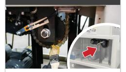
Using the paint brush, dip it in the grease and apply to the chains located on the front of machine.
