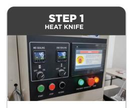
Turn on the machine and let the machine heat up.
