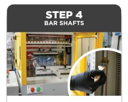
Check seal bar shafts, if dry apply a light coating of grease.
