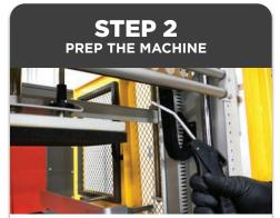
Blow air around the machine using compressed air, paying special attention to all moving parts.
