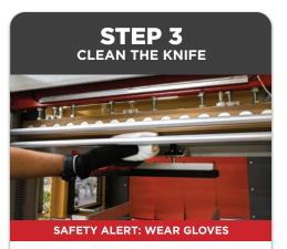
After the knife has heated up, check knife of any plastic residue. If residue is present, wipe down the hot seal bar with a clean cloth.
