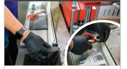
Measure and apply the Teflon tape to seal pad.
