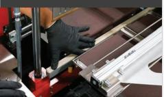
Once Teflon is applied, reattach the sealing pad in its original position.
