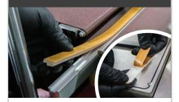
Check the condition of your Teflon tape. If burnt, it will need to be replaced.
