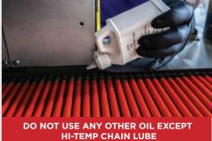
Apply the lube to the chain evenly and continuously until the chain completes a full rotation.
