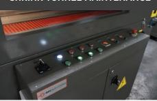
If you have a shrink tunnel connected, turn on the shrink tunnel and increase the conveyor speed to maximum.
