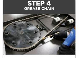
Use a paint brush and dip it in all purpose grease. Apply the grease to the turntable chain.
