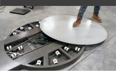
Using your foot, slide turntable back on to the base of the machine.
