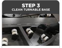
Using compressed air, blow out all residue and trash that is in the turntable base.
